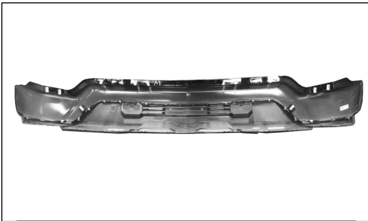
(Fig 20) Separate bottom plastic bumper from upper piece
