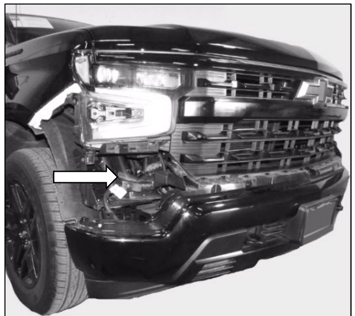
(Fig 4) Remove fascia body panel. If vehicle is equipped with front parking sensors/fog lights, disconnect the bumper harness on the passenger side
