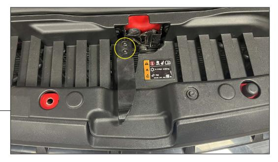
Open the vehicle hood. Remove (2) T-15 Torx bolts from the hood latch. Remove the hood latch and set aside.
