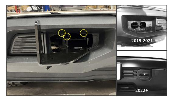
Fit the lower mounting bracket into the vehicle frame where the tow hooks were installed. Then, fit (1) M12 double nut plate and (1) M12 single nut plate through the bracket and vehicle frame. Loosely secure the mounting bracket into place using (3) M12 flat washers, (3) M12 lock washers, and (3) M12 nuts. Repeat this step for the opposite side lower mounting bracket.
