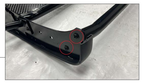
Loosely secure the center support tube to the LH and RH bumper panels using (4) M10 x 30mm Allen bolts, (8) M10 flat washers, and (4) M10 lock nuts.
