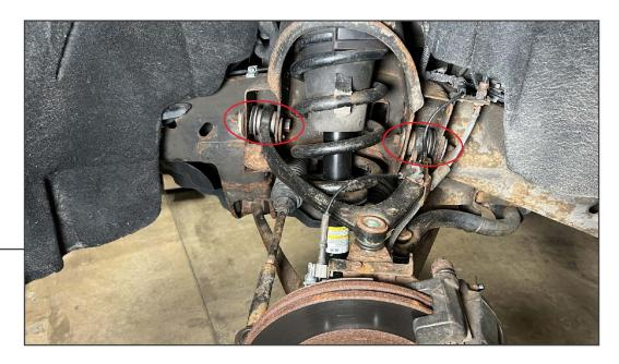
Remove (2) 21mm bolts & nuts from the upper control arm to the vehicle frame. Remove the control arm from the vehicle.
