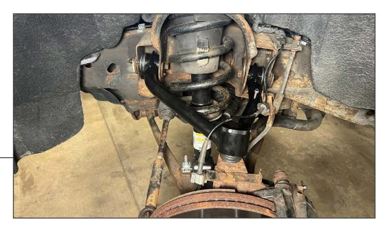
Secure the ball joint to the vehicle steering knuckle using the included (1) 18mm lock nut.
