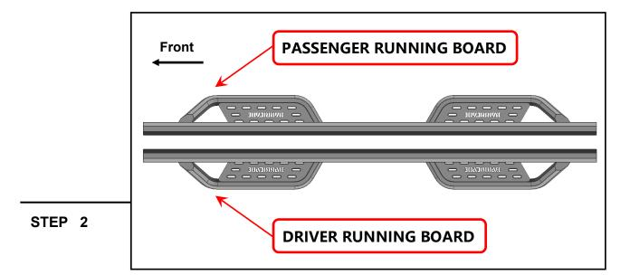
Identify each running board by identifier on the front. Notice: "D" for Driver/Left Side; "P" for Passenger/Right Side.
