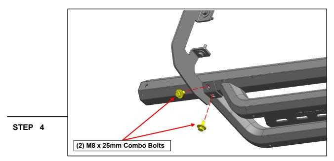
With all brackets loosely mounted to the vehicle, fit the running board onto the brackets, and loosely secure into place using (8) M8 x 25mm combo bolts.
