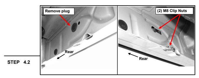
Remove the rubber plug from the larger hole. Slide (1) M8 clip nut into the larger hole. Line up the threaded nut with the smaller hole.
