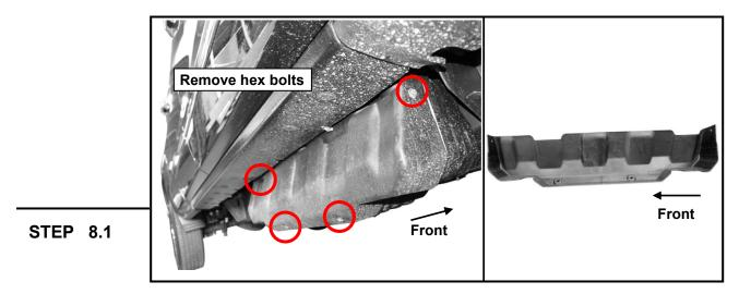
Remove the (4) hex bolts attaching plastic cover to DEF tank and remove plastic cover for better access. **NOTE:** On 2017-on 2500/3500 models, only remove plastic cover from DEF tank. **Do not lower DEF tank** and proceed to **Step 9**.
