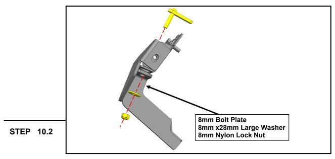
Insert (1) M8 bolt plate down through the hole in the Passenger reinforcement bracket and tab. Loosely connect the (1) Passenger Front step bracket to the bottom of the body and (1) M8 bolt plate using (1) M8 x 28mm flat washer, and (1) M8 Nylon Lock Nut.
