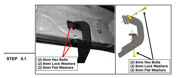
Loosely fit the (1) Driver Front step bracket to the vehicle installed weld nut using (2) M8 x 30mm bolts, (2) M8 lock washers, and (2) M8 flat washers. Do not fully tighten to allow for later adjustments.
