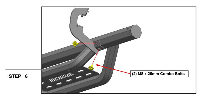
With all brackets loosely mounted to the vehicle, fit the (1) LH Drop Step onto the brackets, and loosely secure into place using (8) M8 x 25mm combo bolts.
