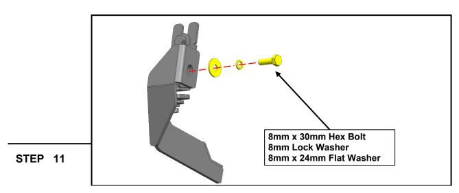
Loosely connect the (1) Passenger Front step bracket to the (1) Passenger reinforcement bracket using (1) M8 x 30mm hex bolt, (1) M8 x 24mm flat washer, and (1) M8 lock washer.
