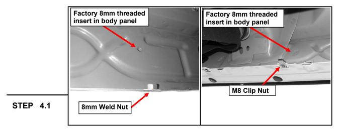
Determine the correct procedure for your model year and each Bracket location.
