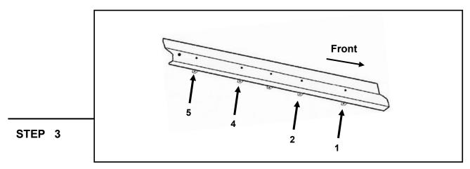
Start installation toward the front of the Driver/Left side of the vehicle.
