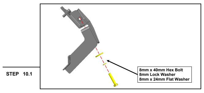
Slide the Bracket over the weld-nut. Loosely connect the (1) Passenger Front step bracket to the bottom of the body and weld-nut using (1) M8 x 40mm hex bolt, (1) M8 x 24mm flat washer, and (1) M8 lock washer.
