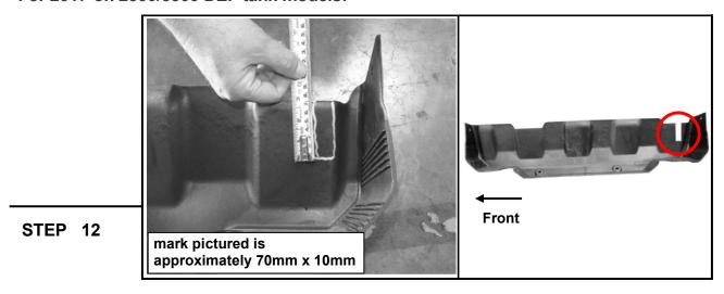
Locate the 2nd mounting location along the bottom edge of the body. Hold the DEF cover in place and mark the 2nd Bracket location onto the cover. Use a sharp knife or hacksaw blade to carefully cut a slot in the plastic cover to clear the 2nd Bracket. Remove as little plastic as possible
