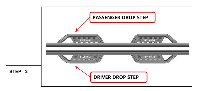
Identify each drop step by identifier on the front. Notice: "D" for Driver/Left Side; "P" for Passenger/Right Side.
