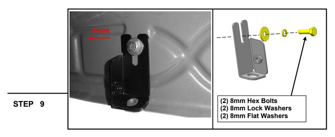
Locate the first tab on the edge of the pinch weld. Repeat **Steps 4 & 5** to attach the (1) Passenger Front reinforcement bracket to the side of the rocker panel. Do not fully tighten to allow for later adjustments.
