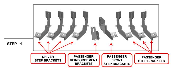
Mounting Brackets per side are the same. Please identify each mounting bracket using the engraved location identifier. Notice: The Passenger/Right Front Mounting location will use front step bracket and reinforcement bracket.
