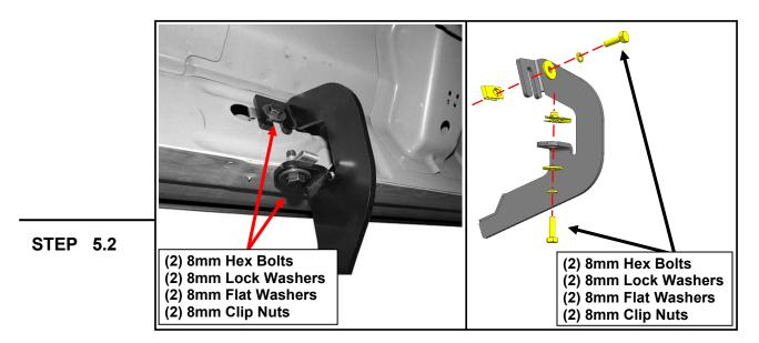
Loosely fit the (1) Driver Front step bracket to the vehicle threaded body hole using (2) M8 x 30mm bolts, (2) M8 lock washers, (2) M8 flat washers, and (2) M8 clip nuts. Do not fully tighten to allow for later adjustments.
