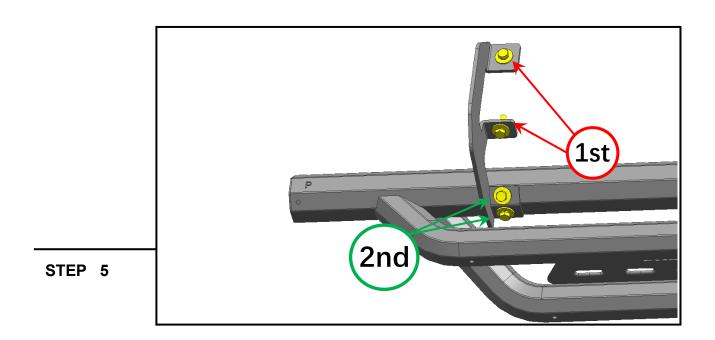
Tighten the mounting brackets to the vehicle. Adjust the Drop Step to the desired angle, and tighten the M8 combo bolts to secure the step into place. See photo for tightening order visual.
