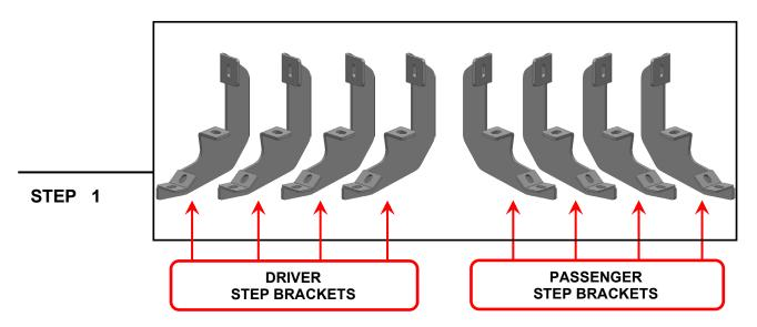
Please identify each mounting bracket using the engraved location identifier. Notice: The brackets can be used at any position along the same side of the vehicle.
