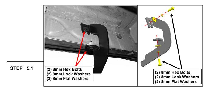
Loosely fit the (1) Driver Front step bracket to the vehicle installed weld nut using (2) M8 x 30mm bolts, (2) M8 lock washers, and (2) M8 flat washers. Do not fully tighten to allow for later adjustments.
