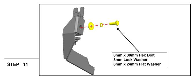
Loosely connect the (1) Passenger Front step bracket to the (1) Passenger reinforcement bracket using (1) M8 x 30mm hex bolt, (1) M8 x 24mm flat washer, and (1) M8 lock washer.
