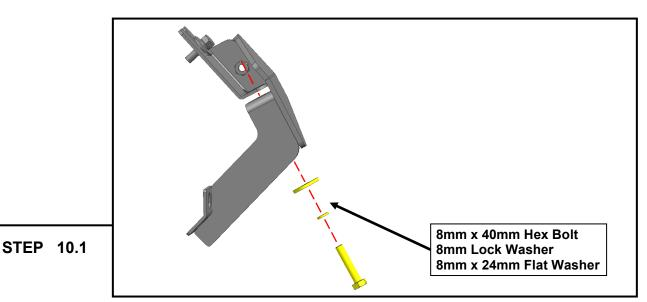
Slide the Bracket over the weld-nut. Loosely connect the (1) Passenger Front step bracket to the bottom of the body and weld-nut using (1) M8 x 40mm hex bolt, (1) M8 x 24mm flat washer, and (1) M8 lock washer.
