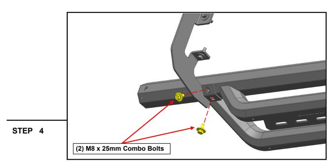
With all brackets loosely mounted to the vehicle, fit the Passenger/Right Drop Step onto the brackets, and loosely secure into place using (8) M8 x 25mm combo bolts.
