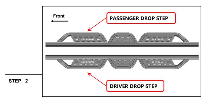
Identify each drop step by identifier on the front. Notice: "D" for Driver/Left Side; "P" for Passenger/Right Side.
