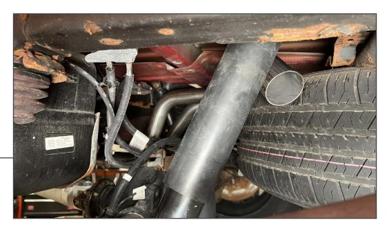
Install the LH over axle pipe to the muffler. Do not fully tighten the exhaust clamp to allow for adjustment later. Fit the over axle pipe into the (1) vehicle rubber hanger.
