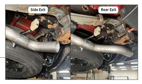
Fit the desired side/rear exit pipe to the vehicle tail pipe. Loosely secure using the previously placed (1) 2.5" exhaust clamp.
