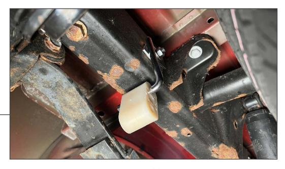
In between the vehicle leaf spring and the frame, mount the (1) exhaust hanger mount to the vehicle frame. Use the (2) square plate washers on each side of the frame, then add the hanger mount onto the inside of the frame. Secure using the included M10 hardware.
