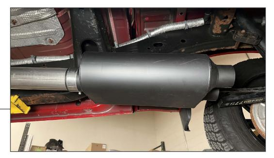
Install the muffler to the front pipe and secure into place using the previously placed (1) 3" exhaust clamp. Do not fully tighten to allow for adjustment later.
