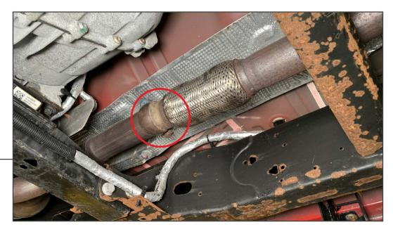
Lift and support the vehicle using a floor jack and jack stands. Locate the front exhaust clamp securing the exhaust system to the catalytic converter. Loosen the clamp using a 13mm socket.
