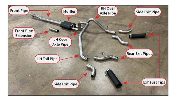
Lay out and identify all exhaust components.
