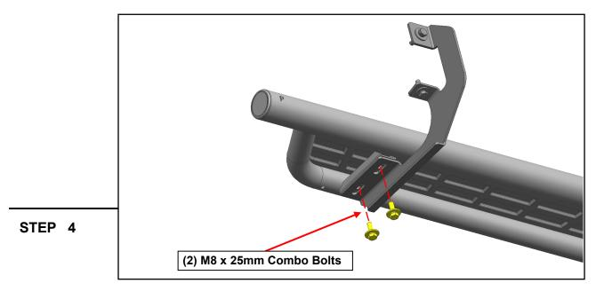
With all brackets loosely mounted to the vehicle, fit the running board onto the brackets, and loosely secure into place using (8) M8 x 25mm combo bolts.
