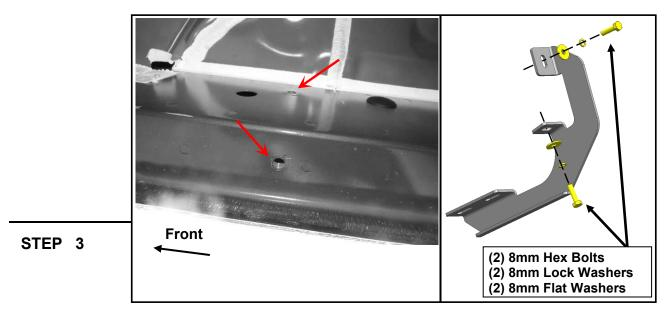
Start installation toward the front of the Passenger/Right side of the vehicle.
