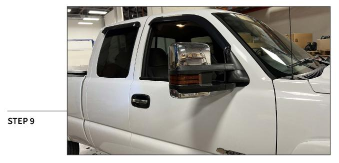
Test all mirror functions, and then install the door panel reusing all original hardware/trim.
