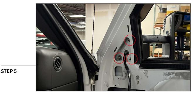
While supporting the original mirror, remove the (3) 10mm bolts and remove the mirror from the vehicle.
