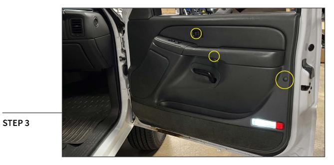
Remove the (1) T-20 Torx bolt along the outside of the door (under the previously removed cap).
