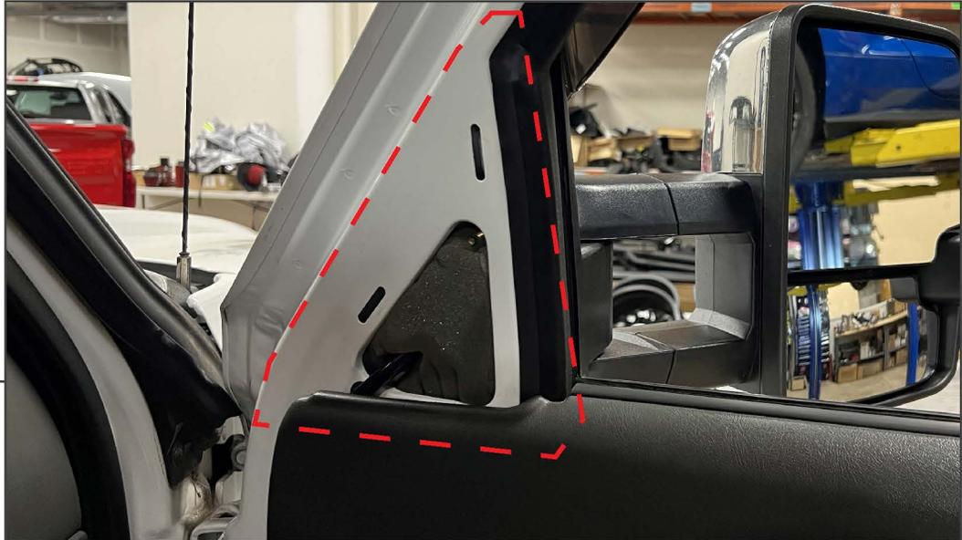
It is recommended to lower the vehicle window before disassembly. Open the vehicle door.
