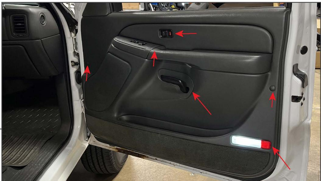
Using a plastic pry tool, remove the following items from the door panel. Set all items aside.
