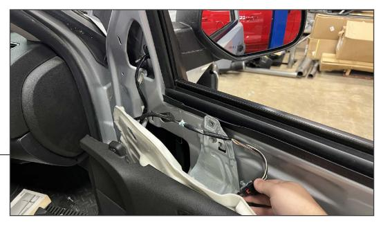
Locate and unplug the mirror harness from the vehicle door harness. Remove any mirror harness retainers from the door.
