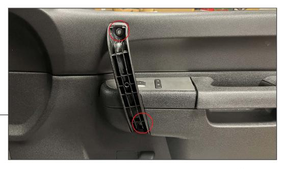
Use a small pry tool to remove the cover around the front grab handle. Then, remove (2) 10mm bolts from the grab handle. Set the grab handle aside.
