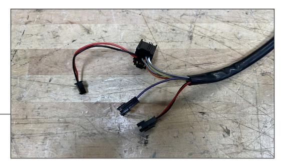
Identify the mirror wiring harness connectors. Depending on vehicle OE equipment, splicing the lighting into the vehicle may be required.
