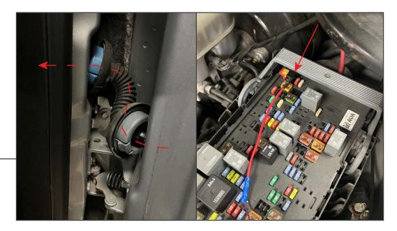
Disconnect the door wiring loom from the chassis and door. Then, use a small flexible wire guide to guide the wire lead into the vehicle cabin.
