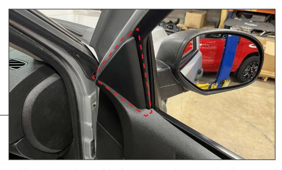
Use a pry tool around the trim along the top of the door panel. Set the trim panel aside.
