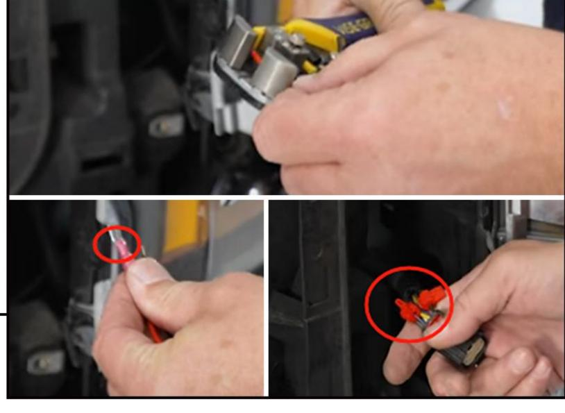
Open the hood, use a trim removal tool to remove 12 push Remove 3 bolts (2 at the top, one at the bottom) on the pins to remove radiator cover. Then take four 10-millimeter passanger side headlight to swing the headlight apart so bolts at the top first, grab the grille at the top and in the middle to pull it away.
