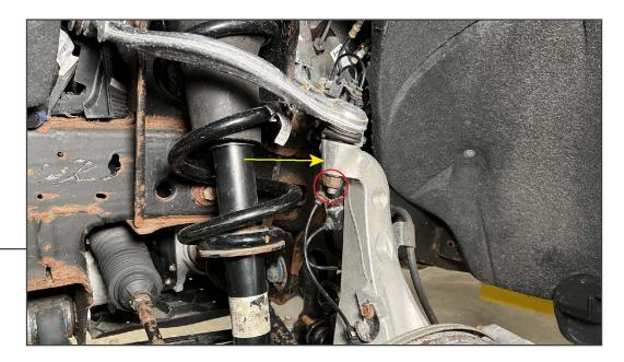
Loosen (1) 18mm nut from the upper ball joint. Then, strike the steering knuckle to dislodge the ball joint from the steering knuckle.
