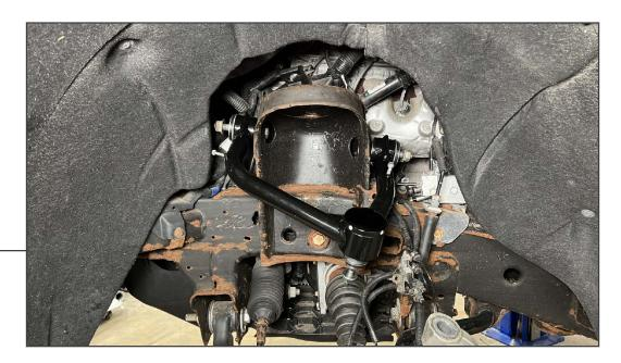
Fit the new control arm to the vehicle using the original control arm hardware. Do not fully tighten the hardware at this time. The control arm mounting bolts will be tightened with the vehicle on the ground with the suspension loaded.
