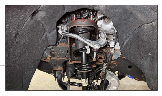
Lift and temporarily relocate the wiring harness away from the upper strut nuts. Then, remove the (3) 14mm strut nuts. Remove the vehicle strut from the vehicle.
