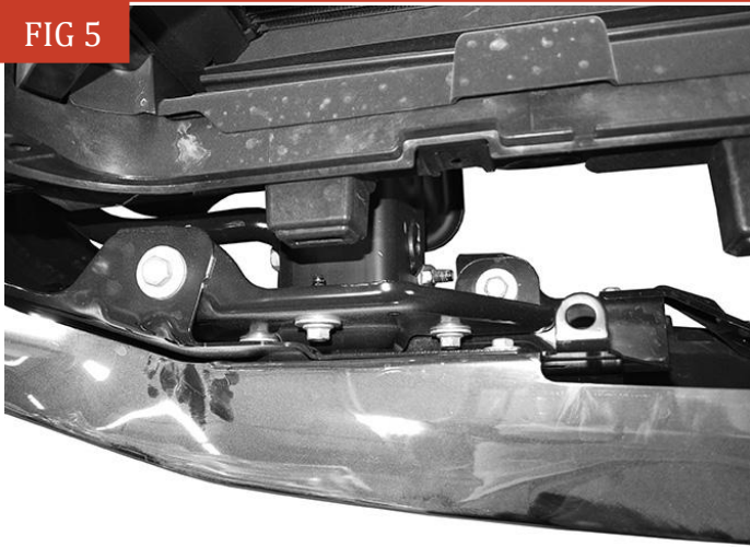
(Fig 5) Remove bumper bolts attaching bumper to brackets- passenger side pictured from above
