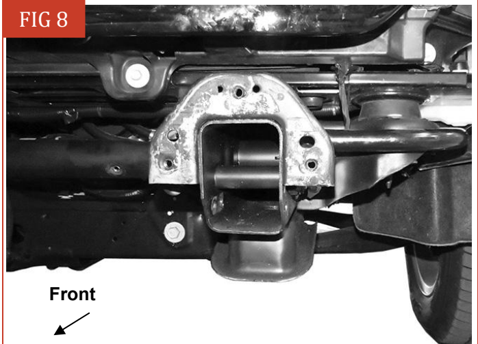
(Fig 8) Example driver/left bumper bracket removed on model without tow hooks
