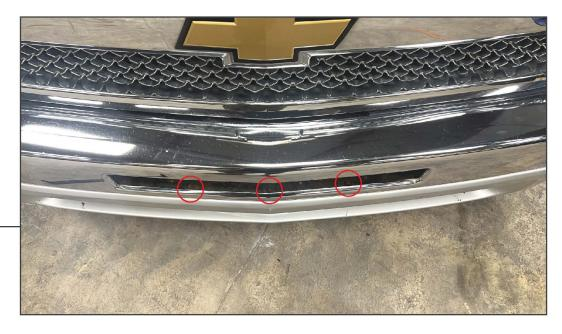
Remove the (3) 10mm bolts from the front bumper slot.
