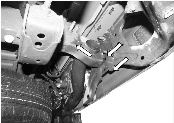
(Fig 2) Factory nuts removed. Bumper Support Bar removed. Reuse the bumper and frame studs (arrows).
