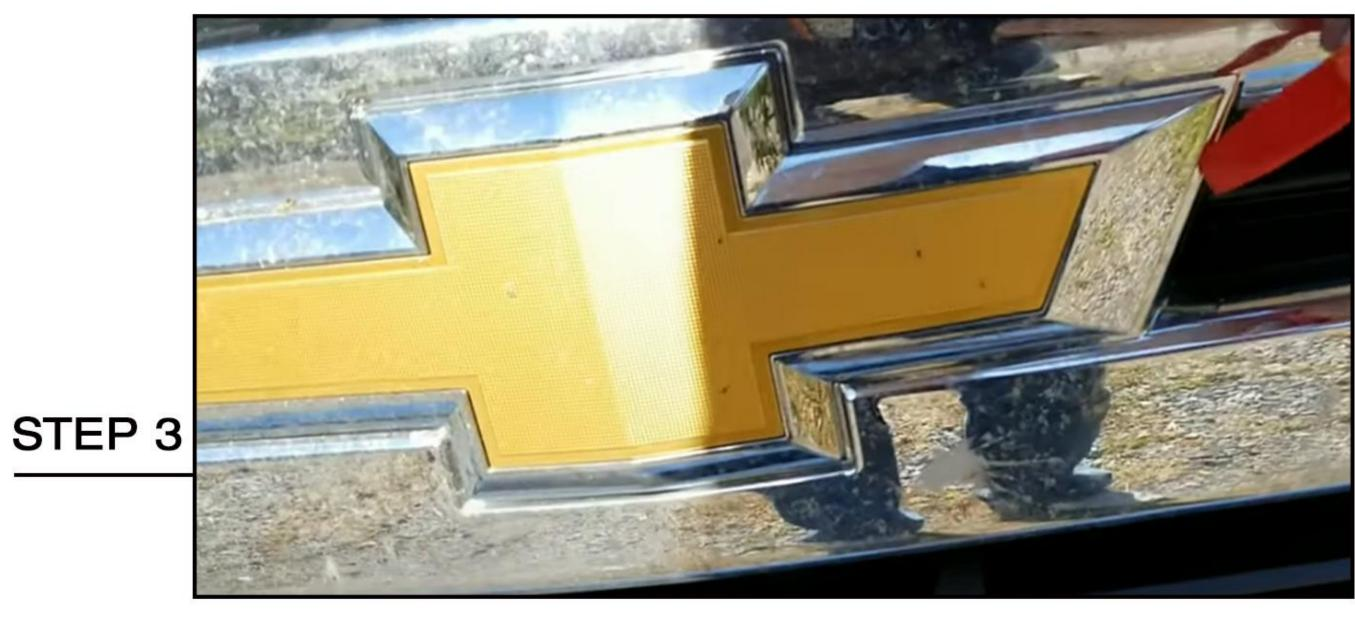
Remove the emblem form the old grille with the trim removal tool and install it on the new grille.
