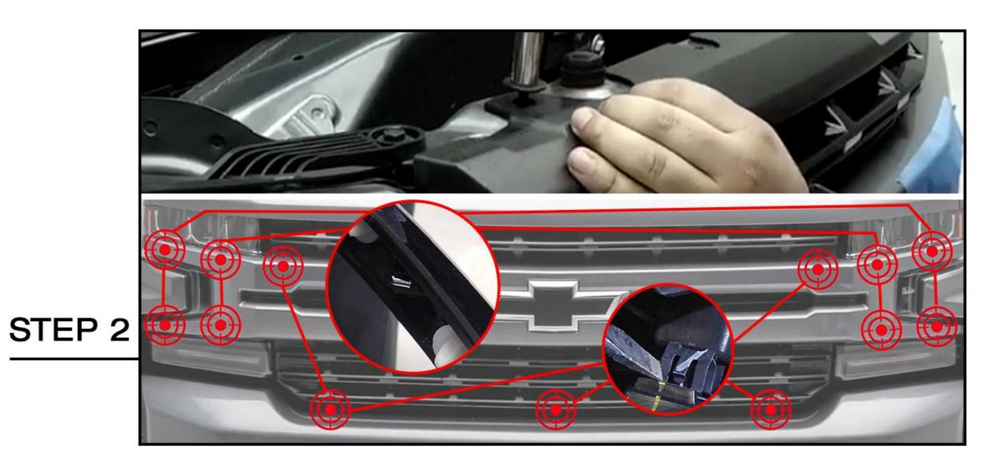
Remove the 4 bolts that hold the factory grille to the frame. Unfasten the remaining clips holding it to the truck: Start with the center bar corners over the headlights, each corner is fastened to the truck with 4 white plastic clips. Release these clips (will be reused) with flat-head screwdriver. Finally pry off the remaining metal clips that run along the edge of the center portion of the factory grille. With all clips unfastened from the truck, remove the grille and place it facedown.
