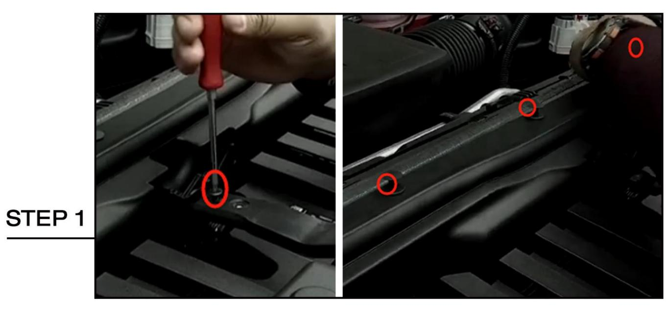
Open the hood,remove the 2 Torx screws attaching it to the hood latch to remove the hood latch handle. Remove the radiator cover by removing the plastic retaining clips.
