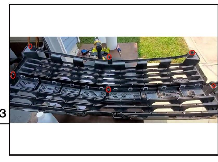
Open the hood, remove the 2 Torx screws attaching it to the hood latch to remove the hood latch handle. Remove the 8 plastic retaining clips to take the the radiator cover out of the car. Remove the four 10 millimeter, then gently pull the grille outward to remove the old grille.
