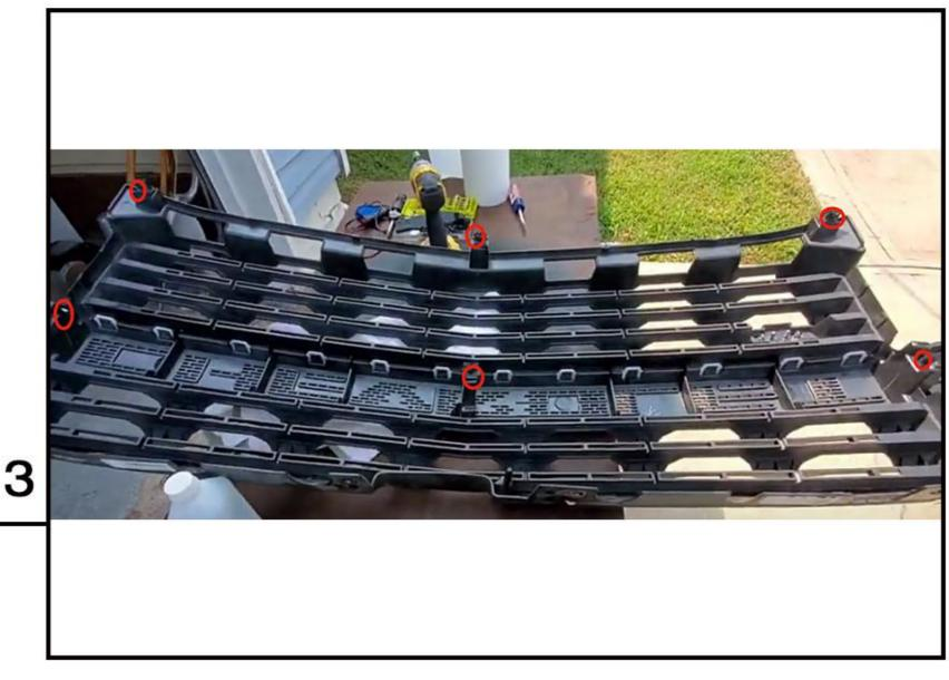
Open the hood, remove the 2 Torx screws attaching it to the hood latch to remove the hood latch handle. Remove the 8 plastic retaining clips to take the the radiator cover out of the car.
