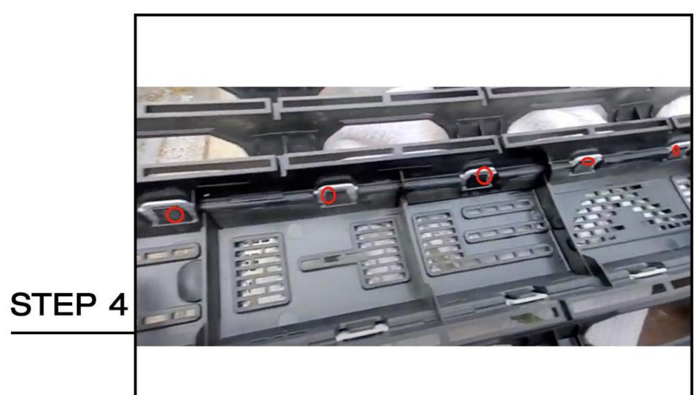
Remove the crossbeam from the original grille and install it onto the new grille.
