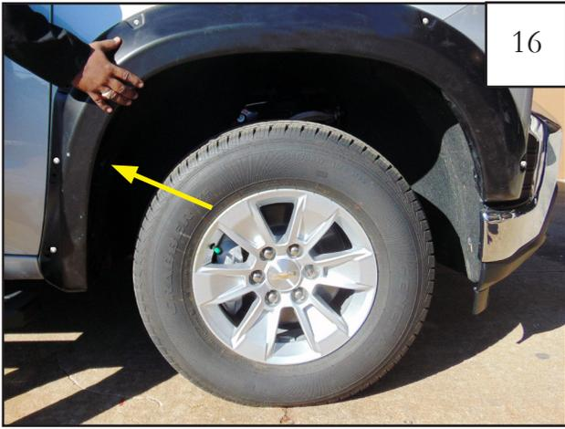
Install (1) supplied phillips head screw (SW1-0058) at rear Clip location. *Do not tighten.* (If needed use an awl to align flare mounting holes.)
