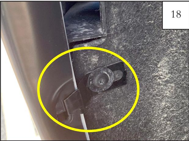
**FOR 2022 ONLY:** Remove (1) T-15 torx screw and install (1) 122441 Clip. Reinstall screw and tighten.
