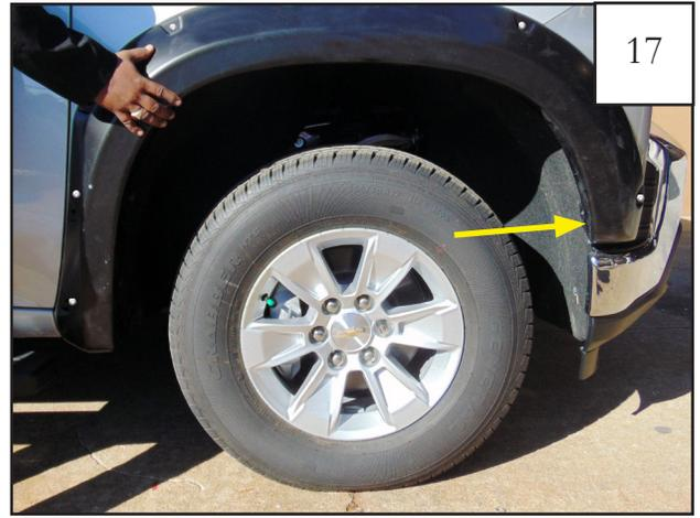
**FOR 2019-2022 LTD ONLY:** Install (1) supplied phillips head screw (SW1-0049) at front Clip location. *Do not tighten.* (If needed use an awl to align flare mounting holes.)
