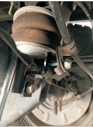
• Relocate hand-brake cable with supplied bracket, 5/16 nut and bolt - refer LH image.
