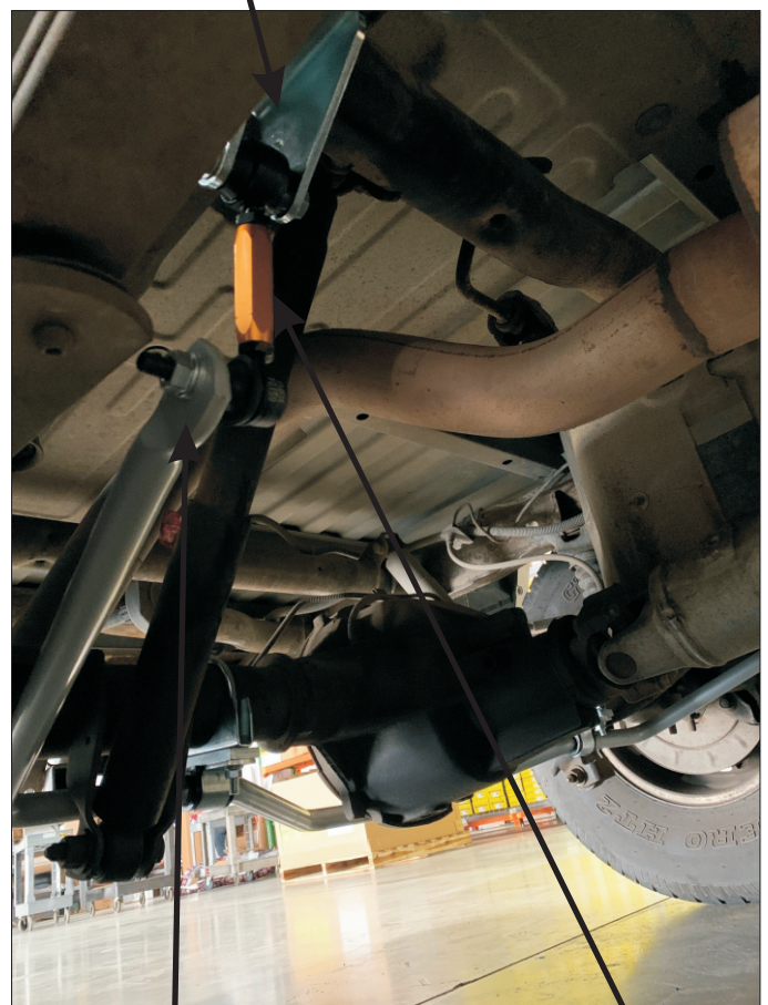
Use flat washers either side of link bushing
