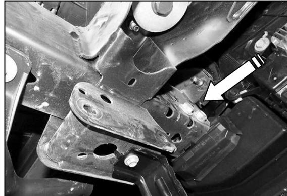
**(Fig 3) Passenger/right outer mounting bolts for tow hook pictured from behind bumper**
