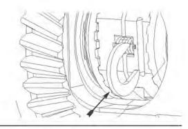
**35.** Making sure drivers stay engaged with couplers, carefully rotate both wheels backwards 1/4 turn to expose pinion shaft opening.
