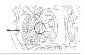
23. Verify spacer paddle is aligned with the paddle opening in synchro ring and press down on driver/spacer to seat on coupler; driver teeth should be fully engaged all the way around.
