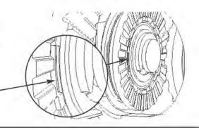
17. Insert the non-slotted spacer into the non-slotted driver. Seat
