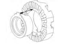
18. Insert driver/spacer as shown, making sure spacer paddle is facing out towards you.
