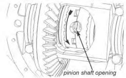
**36.** Feel through pinion shaft opening and verify both spacers and drivers are fully seated onto couplers. Verify all 8 saddle springs are fully seated in holes.
