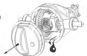
7. Expose pinion shaft; remove retaining bolt/roll pin and shaft.
