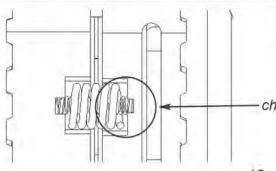
**27.** Visually inspect notches in spring slot to make sure inner spring is fully seated.
