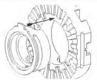
**20.** Insert the slotted spacer into the slotted driver. Seat the spacer paddle at the paddle opening in driver (missing extended tooth).
