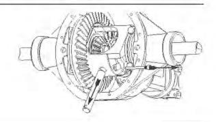
**8.** Push both axles inward and remove both c-clips. Remove orings from c-clip grooves on axle shafts if present.
