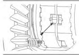
**26.** Compress inner spring and install spring assembly into spring slot.
