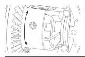
**37.** Keeping couplers and drivers stationary, rotate case 1/4 turn forward to align pinion shaft opening with driver saddles.
