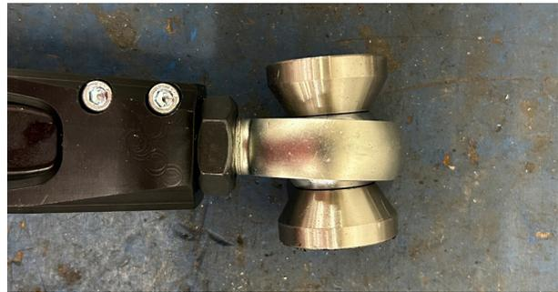
Fig. 14: Install misalignments.
