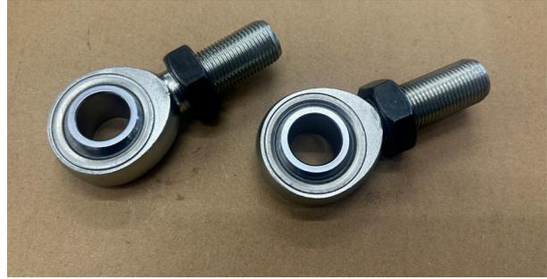
Fig. 10: Install the 3/4" jam nuts.
