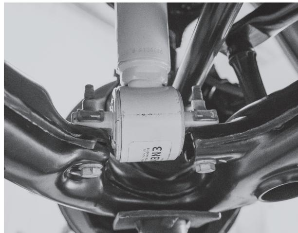
Fig. 6: Remove 2 bar pin bolts.
