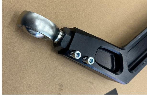
Fig. 13: Loctite and install pinch bolts.
