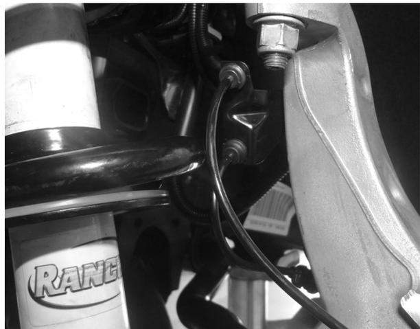
Fig. 4: Unclip ABS wire.
