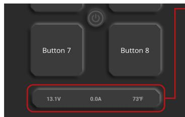
At the bottom of the screen, the status bar displays key information, including vehicle voltage, total output current, and the Hub's circuit board surface temperature.
