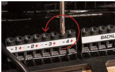
1. To connect an output lead to one of the terminals, use a Phillips screwdriver to open the screw terminal by rotating it counter-clockwise.
