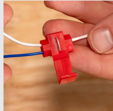
2. Using a quick splice connector, place the sensor wire into the "stopper" end or inner groove of the quick splice connector. Then take the program function wire and place it into the outer groove of the quick splice connector.
