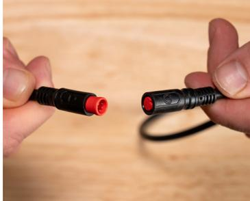
1. Connect the Accessory Harness (sensor wires) to the Hub Harness.
