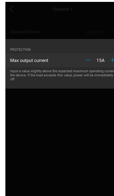
**Max Output Current:** This setting determines the threshold at which the output channel will automatically turn off to protect both the channel and the connected device.
