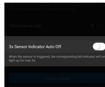
**3s Sensor Indicator Auto Off:** Configures the D-Switch to automatically turn off the sensor wire indicator located on top of the Controller after 3 seconds.
