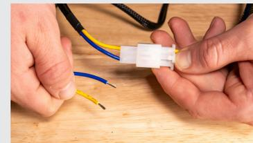
1. Using the included aux-adaptor, replace the toggle switch and connect the leads to the D-Switch terminals.
