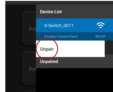
2. In the Device List, the Device ID will appear under the Device List section with a signal indicator next to it. Press and hold the Device ID until a sub-option appears. Then select Unpair.
