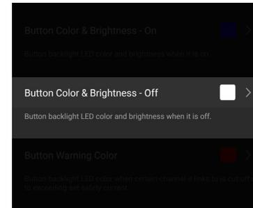
**Button Color & Brightness - Off:** These settings allow you to configure the backlight color and brightness levels when a button is in the Off state.
