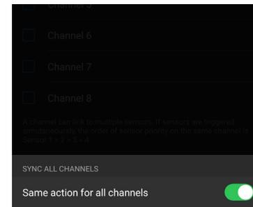
**Sync All Channels:** Enabled by default. When disabled, this function allows users with multiple linked channels to choose a different action for each channel individually.
