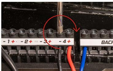
3. Insert the wire into the screw terminal and tighten by rotating the Phillips screwdriver clockwise until it is snug. Gently pull on the wire lead to test that it is secure.
