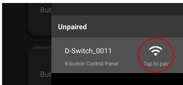
3. In the Device List, the Device ID will appear under the Unpaired section with a signal indicator next to it. Tap the signal indicator to pair the device.
