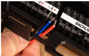
2. Feed the channel leads through one of the openings on the bottom of the Hub base.
