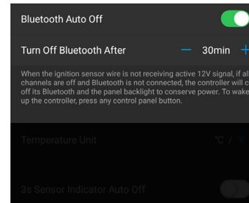
**Bluetooth Auto Off:** When the app is not connected to the controller, all channels are in the Off state, and no 12V is present on the ignition wire, the Bluetooth module and panel will enter sleep mode to conserve power. The panel can be reactivated at any time by pressing any button.
