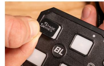
2. Peel off the label and firmly press down on the button.
