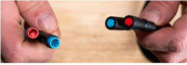
1. Connect the Controller Harness to the included 3-Meter Extension Harness.
