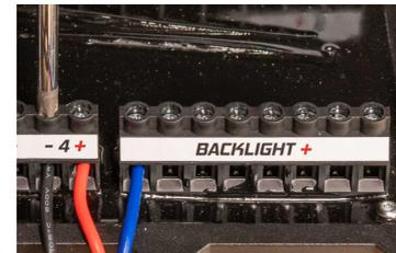
4. If equipped with a backlight, insert the backlight wires into any position on the backlight bus.
