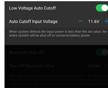
**Auto Cutoff Input Voltage:** The D-Switch continuously monitors the vehicle voltage, which can be viewed on the status bar of the main Control Menu. This option sets the threshold voltage at which the D-Switch will automatically turn off to help preserve the vehicle's battery.
