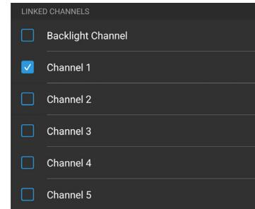
**Linked Channels:** This section links channels (also referred to as outputs) to the button. It's important to note that Button 1 is not fixed to Output 1—any button can be configured to control one or more outputs, including the backlight output.
