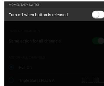
**Momentary Switch:** Disabled by default, allowing the button to toggle On/Off with a single press. When enabled, this setting configures the button to be momentary, meaning the user must hold the button to keep it On. Once released, the button will turn Off.
