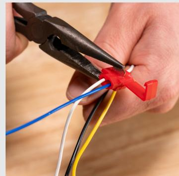
3. Using pliers, squeeze down on the metal part of the quick splice connector. Gently pull on the wires to check that they are secure before closing the connector and locking it in.
