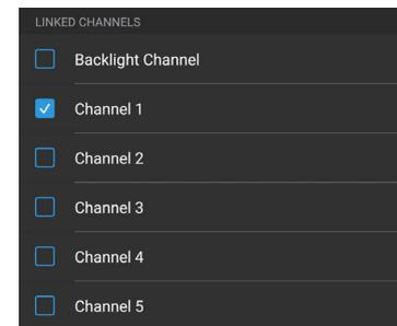
**Linked Channels:** This section links channels (also referred to as outputs) to the sensor wire. Any sensor wire can be configured to control one or more channel outputs, including the backlight output.
