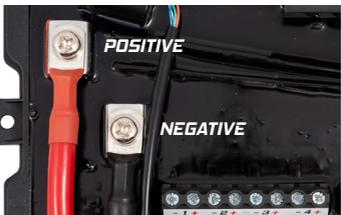
1. Attach the included battery cables (4AWG) to the respective positive and negative terminal blocks.
