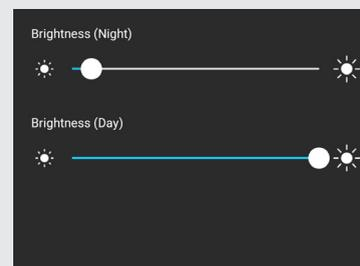
**Button On** and **Button Off** settings each have independent brightness sliders for Night and Day modes. These sliders allow the user to configure the brightness level of the control panel during day and night operation. The control panel will be in Day mode by default. When the **Night Mode** sensor wire detects a +12V, the control panel will switch into **Night Mode**.
