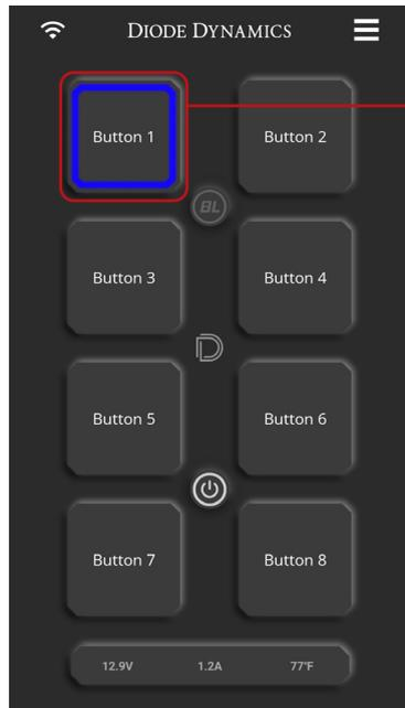
Tapping a button icon will toggle it On/Off. When active, the button's border will highlight to indicate its status.
