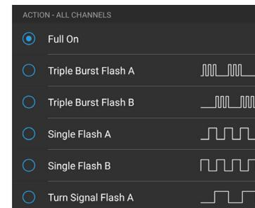
**Actions:** Set to Full On by default. This option allows you to select a Flash or PWM action to be associated with the channel output. When **Sync All Channels** is disabled, an individual selection will be available for each linked channel.
