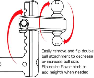
CAUTION!!! Never overload your RAZOR Adjustable Towing System. Weight tested to 10,000 Lbs. NEVER EXCEED WT LIMIT OF YOUR TOW BALL. Always use standard towing procedures and follow supplied check list.
