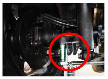
3.Assemble the main body of the traction bar. Raise the Heim End joint up to the Axle Bracket.
