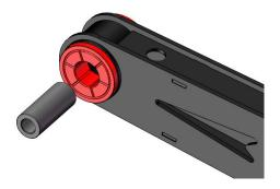
3. Pay attention to the position of the zerk fitting. After installing the kit, screw on the zerk fitting and use a *Lever-Action Manual Grease Gun* to lubricate it.
