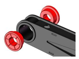
2. Apply **Silicone Based Lubricant** to the tube and press it into the inner hole of the PU bushing.
