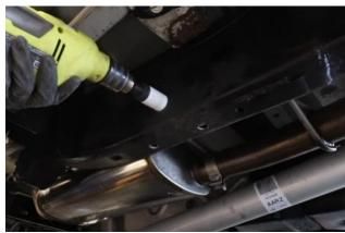
6.Insert the M12 flag nut into the frame from the side and align it with the drilled holes. If alignment is difficult, you can use a 9/16" drill bit to enlarge the hole. A Larger hole size allows for easier adjustment.
