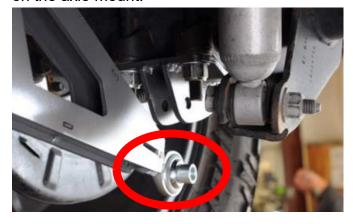
4.Attach the Traction Bar to the Frame Bracket using the supplied M14-90mm bolt and hardware. But do not tighten yet. Mark the location of two holes on the vehicle frame using the frame bracket.
