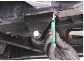
Record the length of the bracket (center to center) to use for adjusting the other side.
