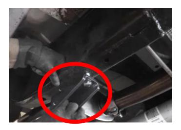
7.Attach the traction bar to the frame bracket using the supplied M14 -90mm bolt and hardware.
