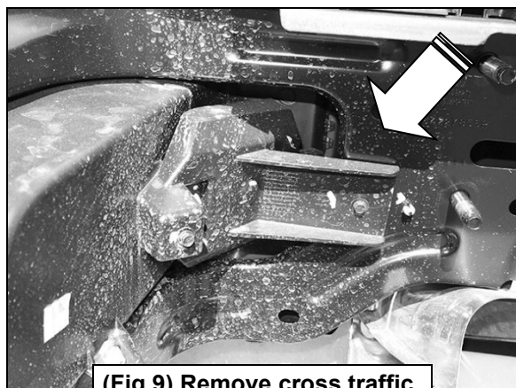
(Fig 9) Remove cross traffic sensors if equipped (arrow)
