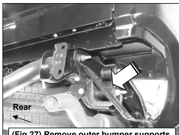
(Fig 27) Remove outer bumper supports from both sides of frame (arrow)
