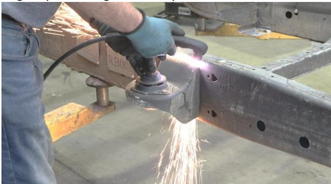
Grind the work area free of rust and debris, revealing bare metal.
