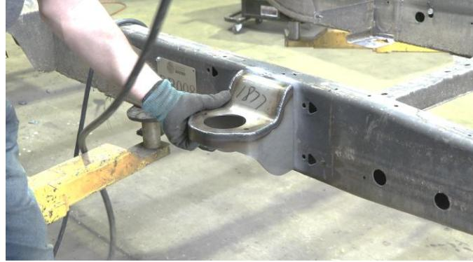
Remove any potential fire hazards from the work area. Following proper welding procedures, tac weld the part onto the frame before welding it on fully. Weld 100% around all edges.
