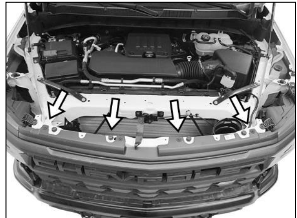
(Fig. 2) Remove hardware attaching grille. Firmly pull grille straight out from vehicle
