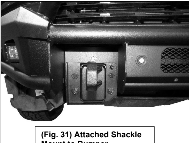
(Fig. 29) Attach Shackle Mount to Bumper and vehicle
