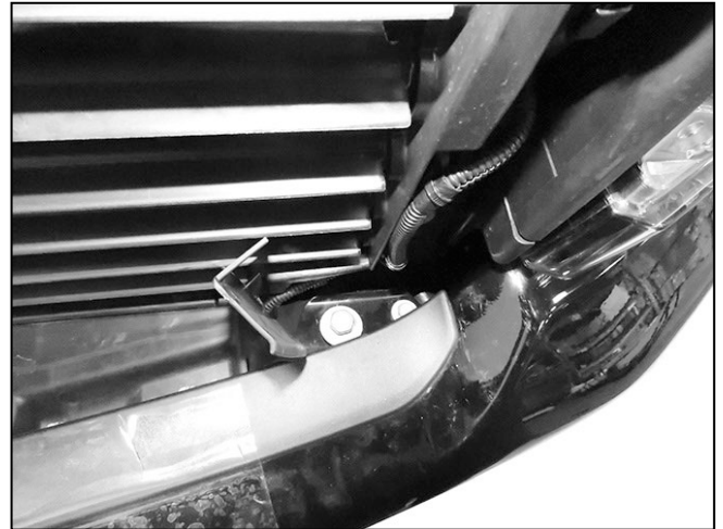
(Fig. 6) Pull back rubber cover to locate bumper bolts
