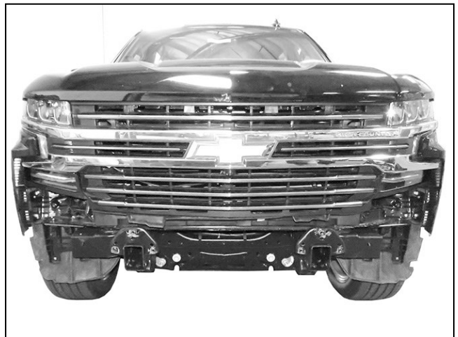
(Fig. 15) Reinstall grille, plastic cover, and hood release handle
