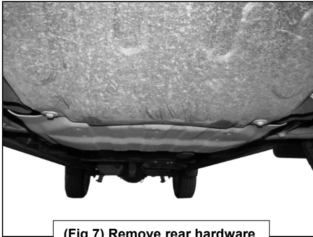
(Fig 7) Remove rear hardware for factory skid plate
