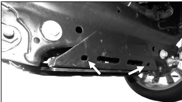
(Fig 9) Locate Rear Mounting Points to attach bottom of Skid Plate.
