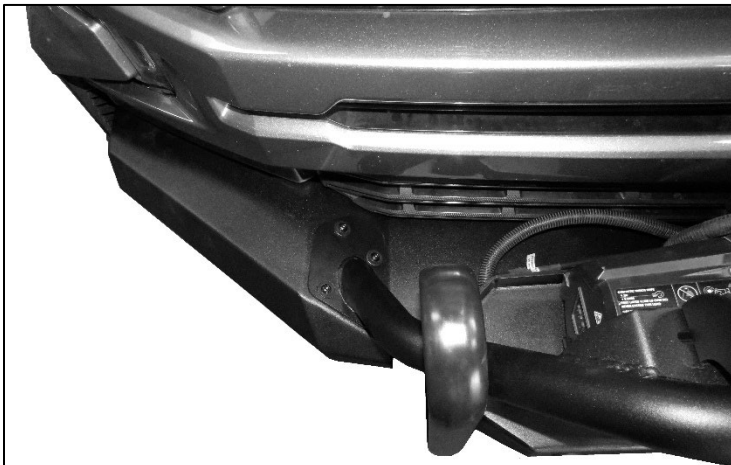
(Fig 10) Attached Passenger/Right Override Tube onto Front Bumper.
