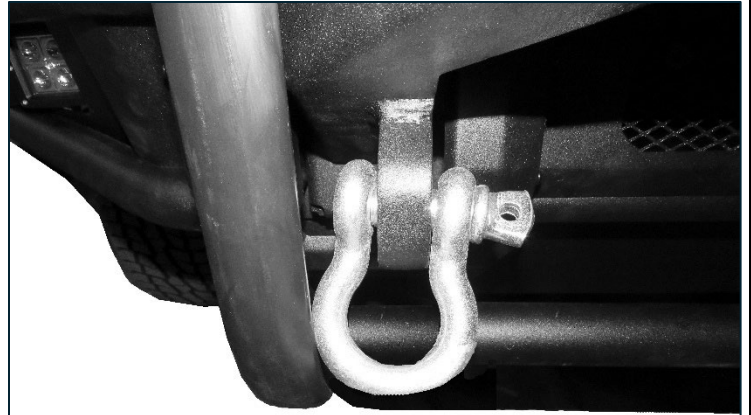
(Fig 14) Attached U — Cover Plate on Passenger/right side and repeat on driver side. NOTE: Tow hook not included
