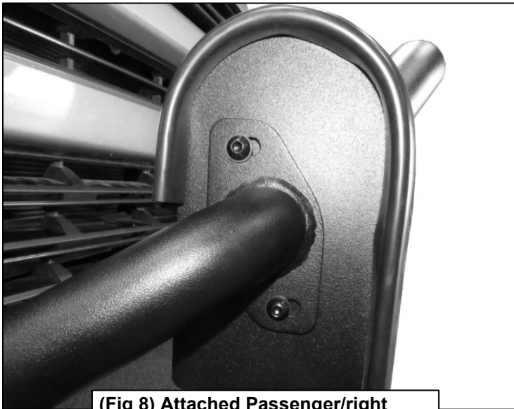
(Fig 8) Attached Passenger/right Override Tube onto HD4 Push Bar.
