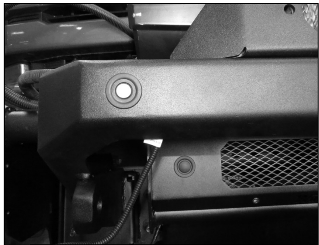
(Fig. 7) Attach parking sensors to Winch Tray and insert Plastic Plugs into Bumper to replace parking sensors
