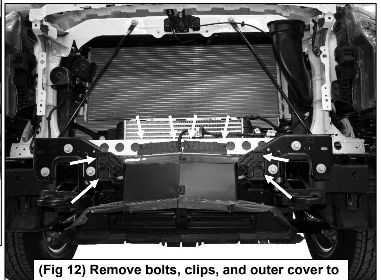
(Fig 10) The cover is held in place by plastic tabs underneath (7 total).
