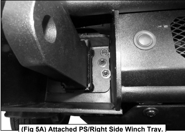
(Fig 5A) Attached PS/Right Side Winch Tray.
