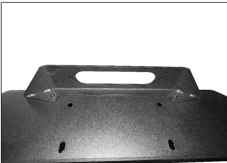
(Fig 3) Attached Fairlead Mount to Winch Tray.
