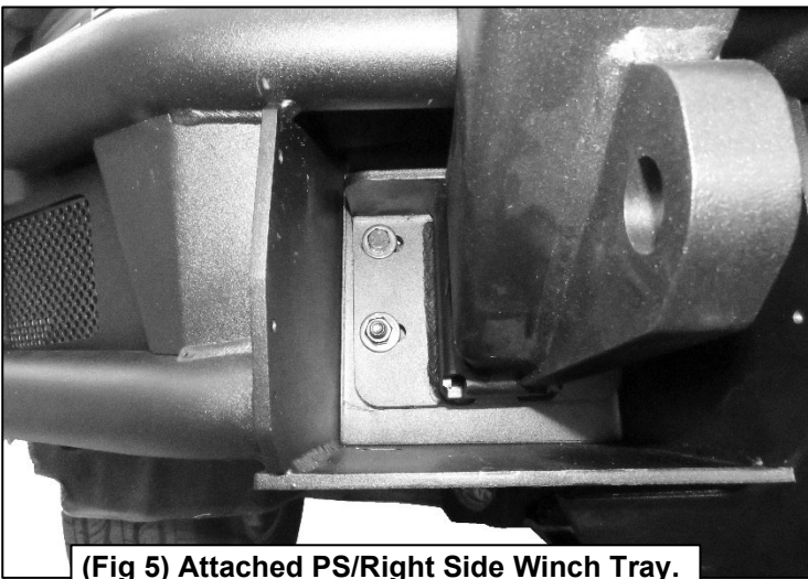
(Fig 5) Attached PS/Right Side Winch Tray.
