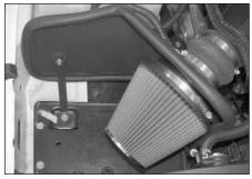
28. Install the Air Filter element onto the intake tube then secure with hose clamp.
