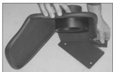
16. Install the trim seal onto the heat shield as shown.
