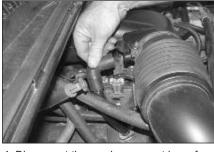
4. Disconnect the crank case vent hose from the factory air intake tube.
