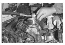
12. Install the aluminum throttle body adapter and hand start the three 6mm bolts.
