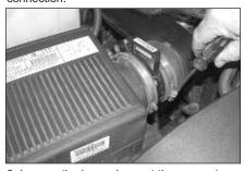
3. Loosen the hose clamp at the mass air sensor as shown.
