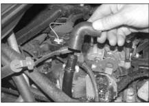
25. Remove the 90 deg rubber hose from the vent tube as shown.
