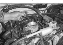
8. Using a 7/32" socket, loosen and remove the factory stud off from the throttle body.
