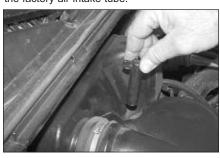
5. Loosen and remove the tall wing nut on the throttle body.
