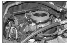
23. Install the silicone hose (08755) over the throttle body adapter and tighten using the provided midi hose clamp.
