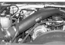
26. Fully install the new K&N intake tube onto the throttle body and mass air sensor as shown. Then tighten the provided hose clamps.
