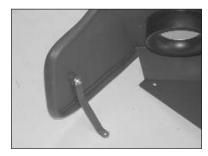
18. Attach the "C" bracket assembly to the heat shield as shown.
