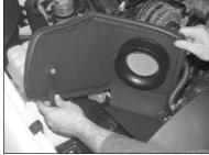
21. Install the heat shield assembly.
