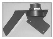
15. Assemble the mass air sensor, heat shield and adapter using the gasket and hardware provided.
