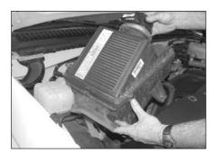
7. Pull firmly upward and remove airbox from vehicle.
