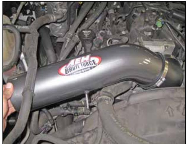
i. Install the intake pipe into the coupler.
