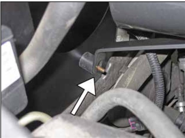
j. Align the bracket with the rubber mount installed in step 3(f).
