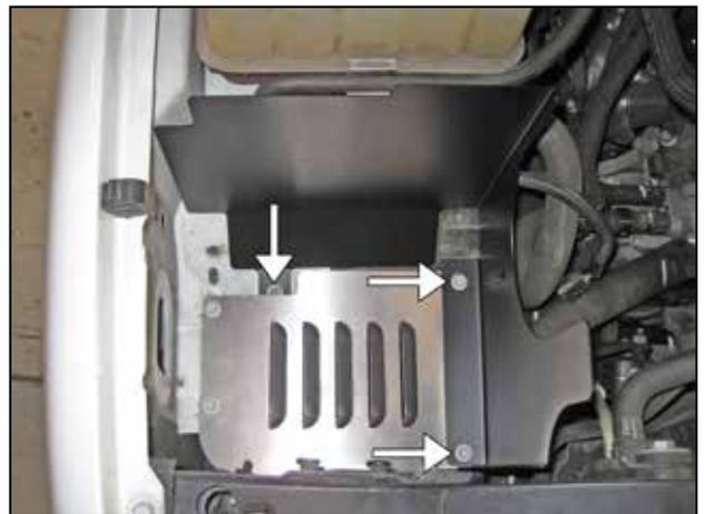
e. Install the 3 remaining stock bolts to secure the heatshield and the splash shield.
