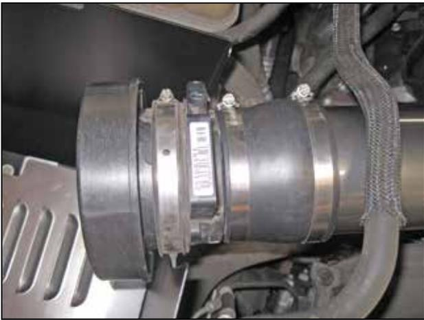
n. Install the MAF sensor assembly (assembled in the previous steps) onto the intake pipe.
