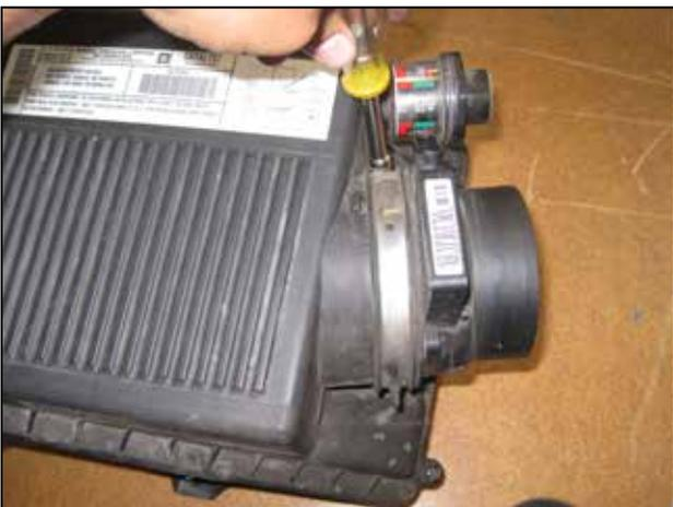
o. Loosen the hose clamp securing the MAF sensor to the stock air box. Remove the MAF sensor from the stock air box.
