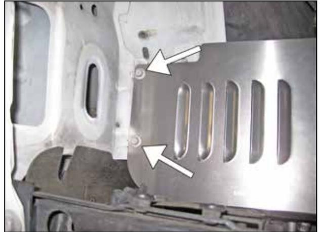
c. Install the two stock bolts to loosely secure the splash shield.
