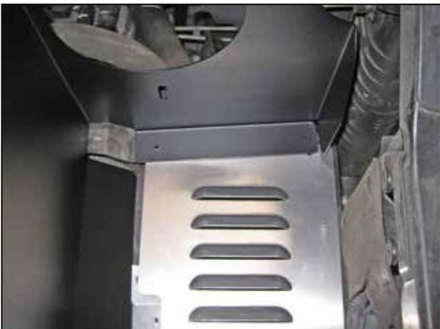
d. Install the heat shield over the splash shield and line up the holes.
