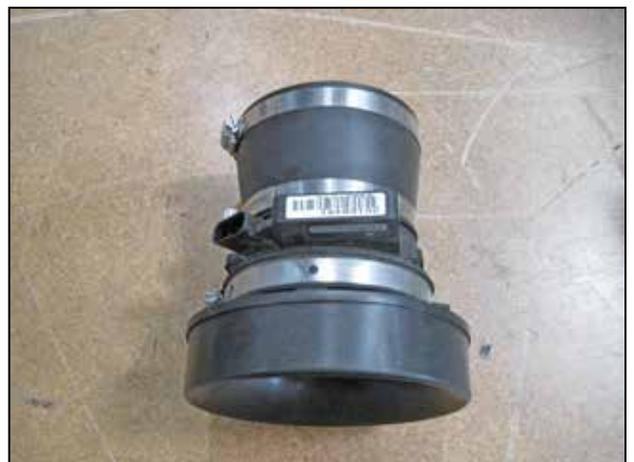
m. Attach the reducer coupler to the MAF sensor and secure with a supplied #64 hose clamp. Loosely attach another #64 hose clamp to the opposite end of the coupler.
