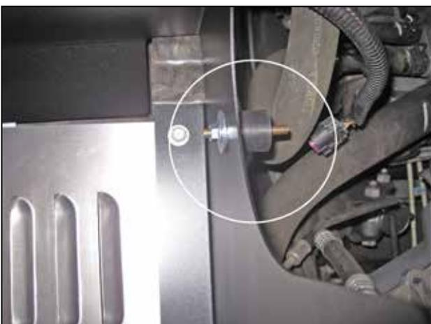
f. Install the rubber mount using the supplied washer and M6 nut on the heat shield.
