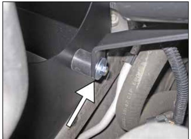
k. Install the supplied washer and the M6 nut.
