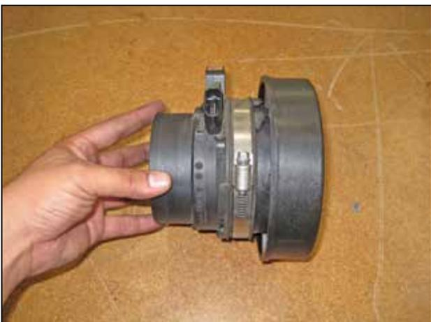
l. Assemble the MAF sensor and the supplied adapter as shown.
