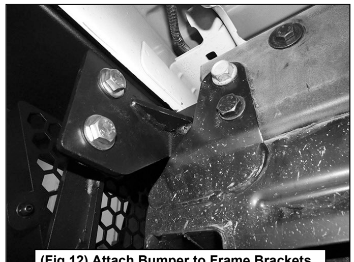
(Fig 12) Attach Bumper to Frame Brackets
