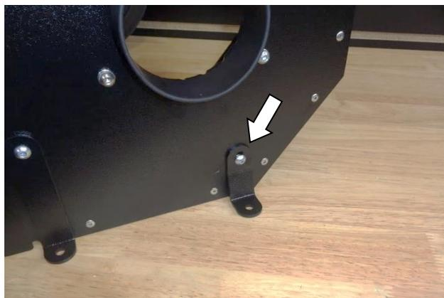
17. Attach short bracket (17) to heat shield using 1/4-20 screw (15) (against the bracket) and nut (21), lock washer (20) and flat washer (19) (against the heat shield). Do not fully tighten hardware at this time.
