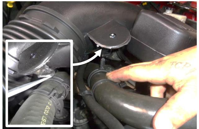
5. Use a flat-tip screwdriver to separate the coolant hose clamp from the intake duct, then remove the clamp from the hose.
