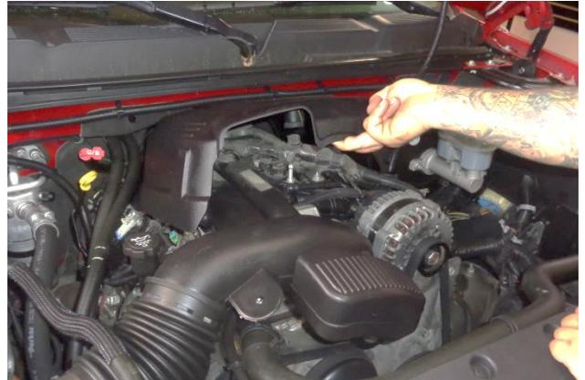
4. Remove the engine cover by firmly lifting it straight up to release it from its friction clips.
