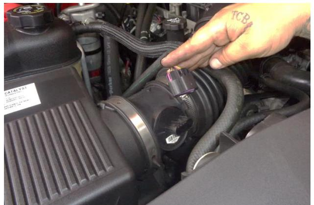
6. Disconnect the electrical plug from the Mass Airflow (MAF) sensor.
