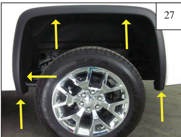
Remove fasteners from factory wheel arch molding using a T-15 Torx Bit for upper and lower wheel well fasteners and a 10mm deep socket and wrench for the lower 2 locations.
