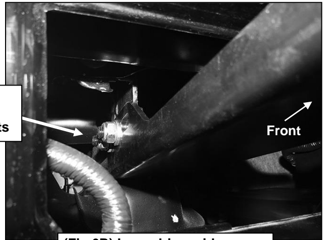
(Fig 6B) Inner driver side Bracket with Double Bolt Plate
