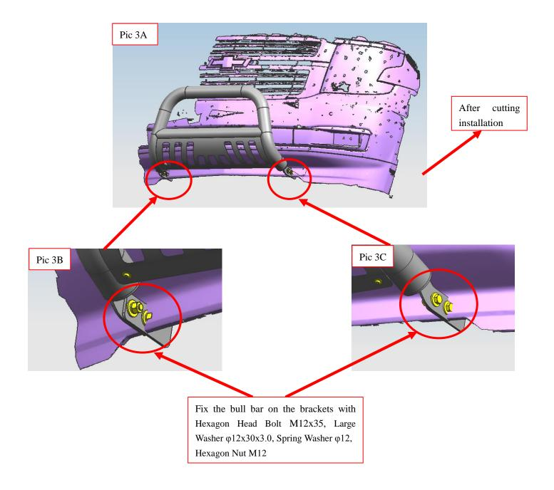
Step 3: Install the bull bar on the brackets and then adjust the brackets to the proper position. Step 4: Check if all hardware are installed and tighten them up to complete the installation.
