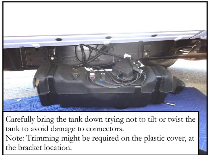
Carefully bring the tank down trying not to tilt or twist the tank to avoid damage to connectors. Note: Trimming might be required on the plastic cover, at the bracket location.
