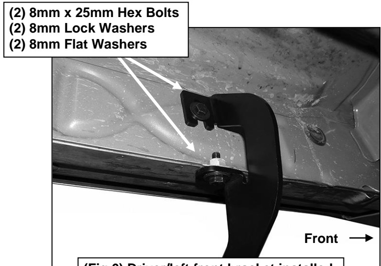
(Fig 6) Driver/left front bracket installed
