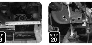
STEP 20: Using a metal cutting device, cut on the line you just made all the way through the bracket. Once separated, debur all rough edges and spray paint.
